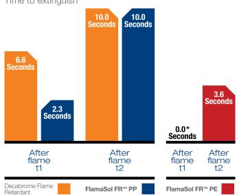
**Protocol:** A torch was used to simulate the UL94 flame test. The flame was held approximately 10mm from a 2 1/2" x 1 3/4" x 1/8" suspended plaque. After burning the part for 10 seconds, the flame was removed. This chart indicates the self-extinguish times. \*No after-flame occurred on flame t1.
